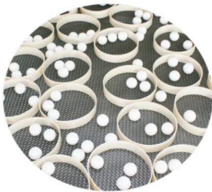
弹跳球清网 Bouncing ball screen cleaning
